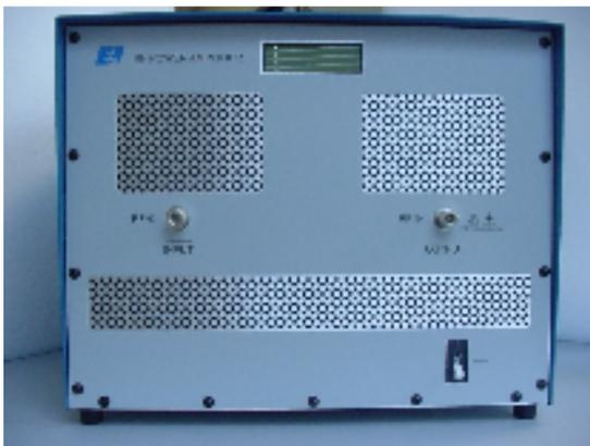
The 1140LA Amplifier is a rugged source of RF power for ultrasonics, induction heating and laser modulation as well as plasma applications. It is a totally solid state solution employing RF DMoS FETs in the power amplification stages, offering simultaneous forward and reverse power readouts, and RS232 port for data collection. The 1140LA reflects E&I's commitment to reliable and robust RF power.
